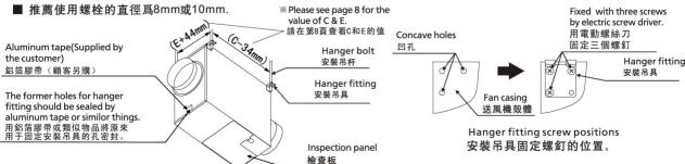
Hanger fitting positions for installing with the inspection panel facing down. 檢查板向下安裝時安裝吊具的位置。
